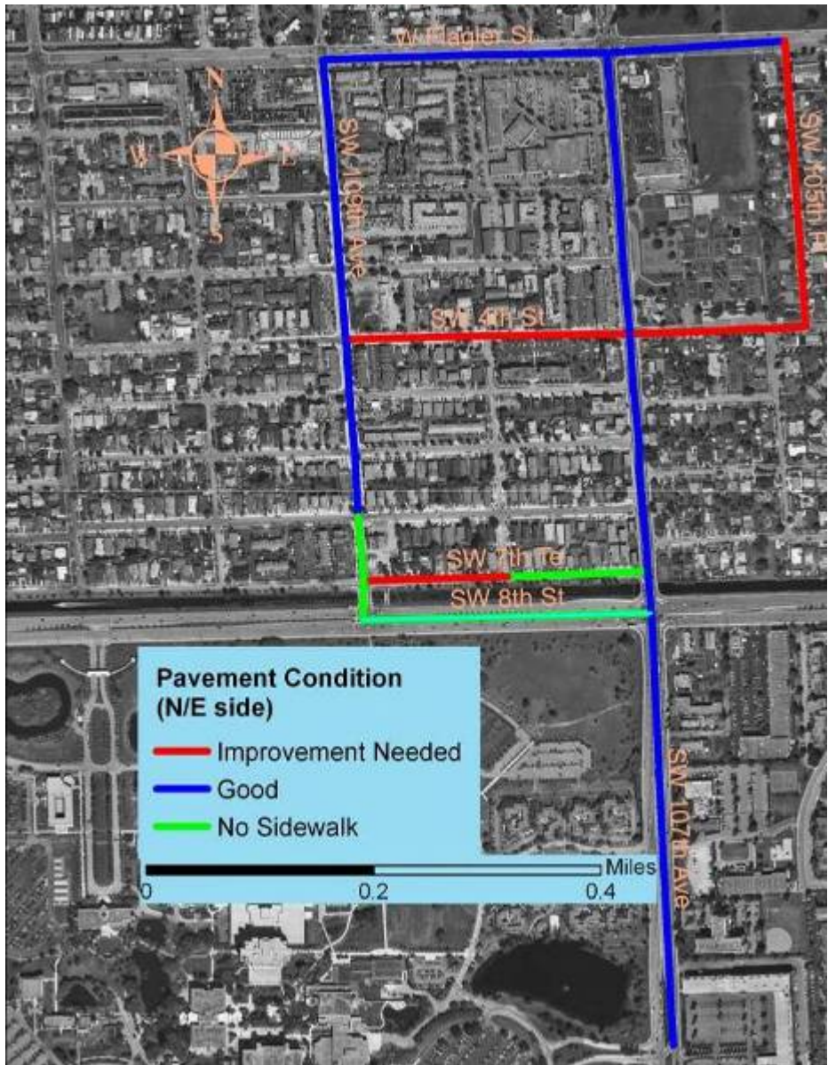
Figure 7.5 Pavement Conditions on North and East Sides of Streets
